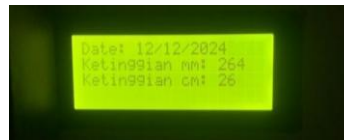
Figure 8. I2C LCD display when the system is turned on
