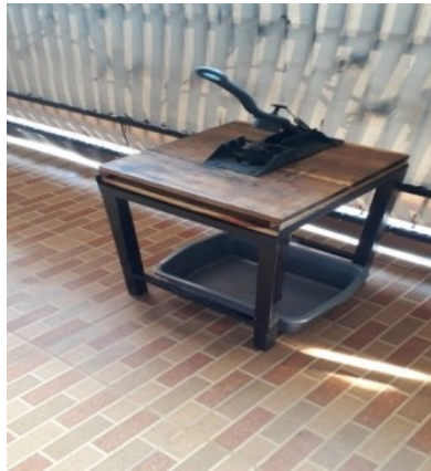
Gambar 2. Alat pengupas jengkol semi mekanis
