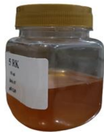
Figure 1. Oil palm liquid sugar processed using lime and evaporated using vacuum rotary
