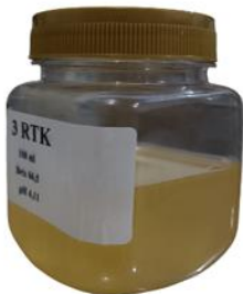
Figure 2. Oil palm liquid sugar processed without lime and evaporated using vacuum rotary
