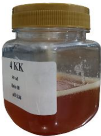
Figure 3. Oil palm liquid sugar processed with lime and evaporated at atmospheric condition
