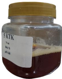
Figure 4. Oil palm liquid sugar processed without lime and evaporated at atmospheric condition
