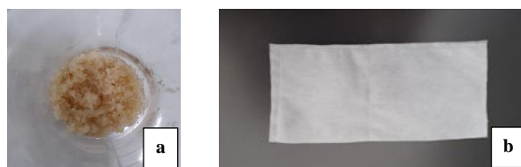
Figure 1. Illustration of the SWA/EE mixture (a) and its active packaging using PP non-woven bags (b)
