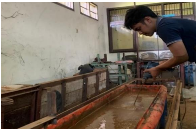
Figure 3. Muddy soil preparation in the soil bin
