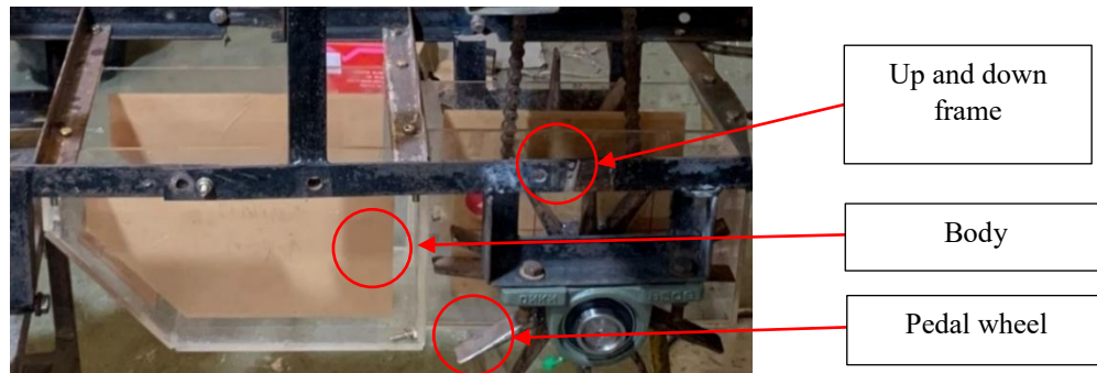
Figure 5 (b). Fabrication results of the pedal-type traction device
