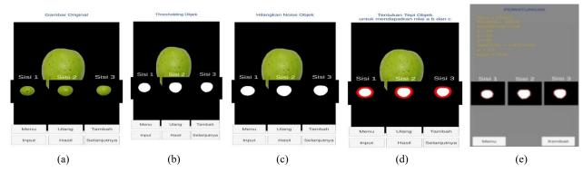
Figure 10. Process display of (a) Grayscale, (b) Thresholding, (c) Removing noise, (a) Object detection process, (e) Calculation result.
