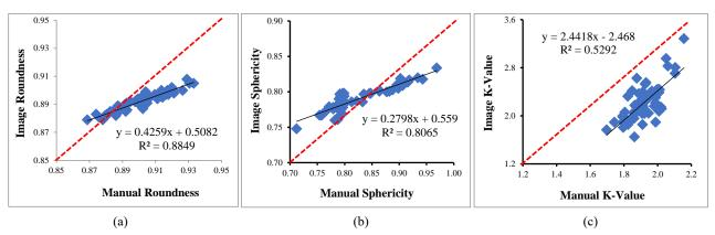
Figure 12. Relation manual calculation and image values of (a) Roundness, (b) Sphericity, and (c) *K* value (dotted red line is for ideal results where image prediction perfectly equal to manual measurement).
