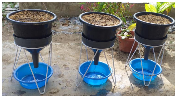
Figure 3. Mechanism for determining field capacity in the planting media used.
