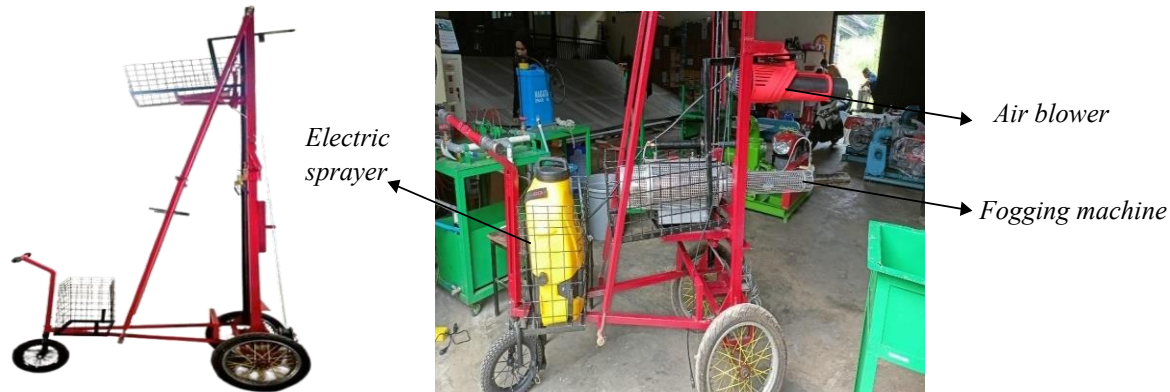
Figure 1. Mobile spray fogger
