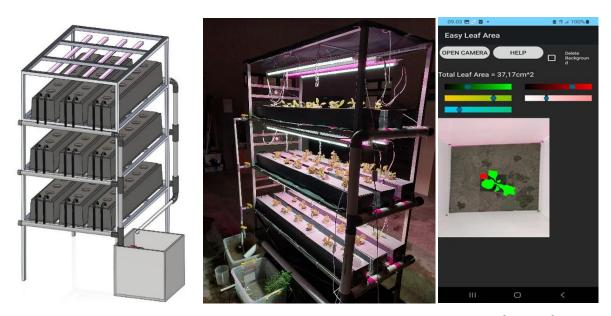
Figure 1. (a & b) Laboratory scale plant factory, (c) Leaf area measurement using Easy Leaf Area software
