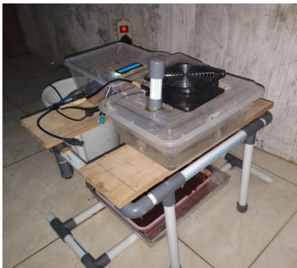
Figure 5. Prototype of the automatic temperature and humidity control device
