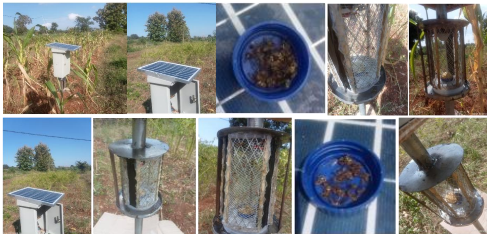
Figure 9. Field testing of fruit fly trap equipment in the cornfield (top) and chili plantation (bottom)
