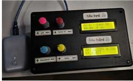
Figure 6. Display of the NPK content from the designed instrument
