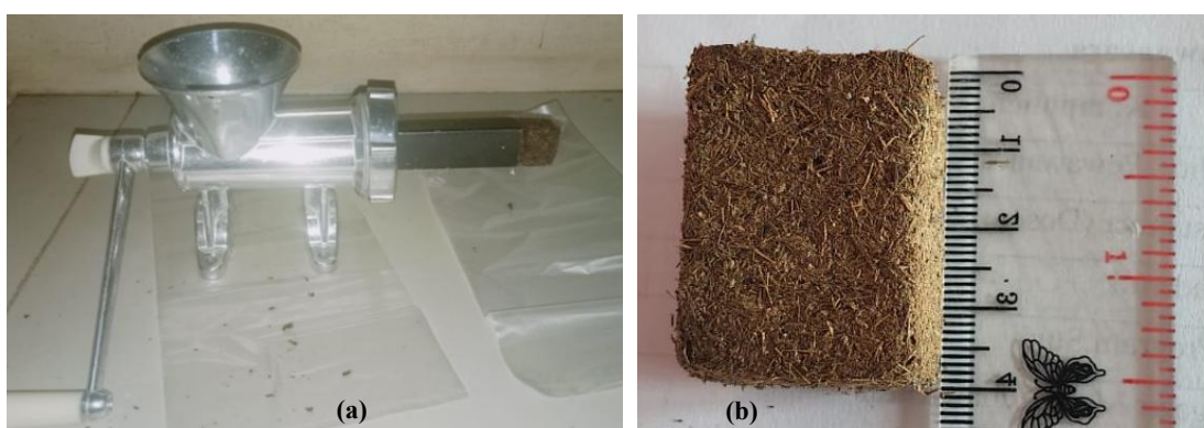
Figure 2. (a) Briquette molding device Type 12, and (b) Briquettes made from banana pseudostem and coconut pulp
