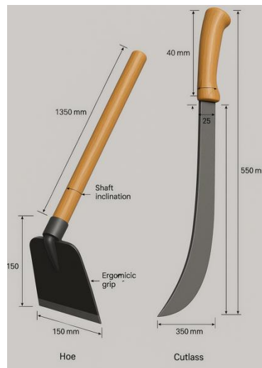
Figure 2. 3D CAD Renderings of ergonomically redesigned hoe and cutlass
