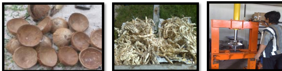
Figure 1. (a) Sun-dry coconut shells, (b) Sun-dry sugarcane bagasse, (c) Briquette compaction process
