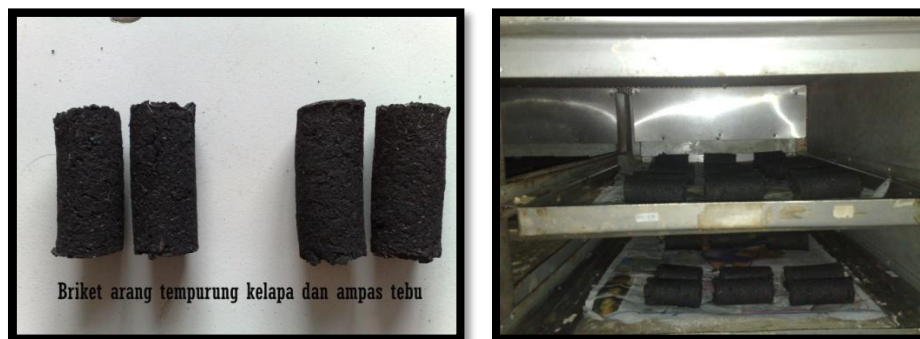
Figure 3. (a) Briquettes made of coconut shell and sugarcane bagasse, (b) Briquette drying
