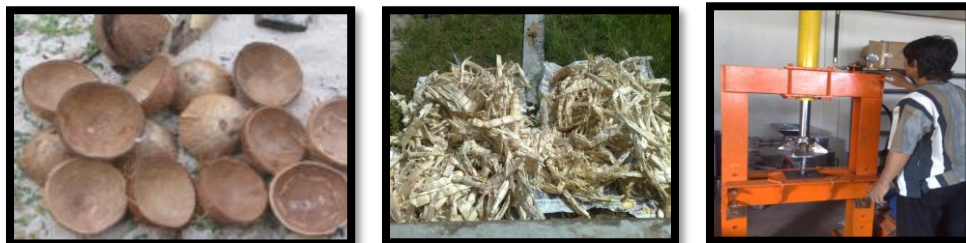
Figure 1. (a) Sun-dry coconut shells, (b) Sun-dry sugarcane bagasse, (c) Briquette compaction process
