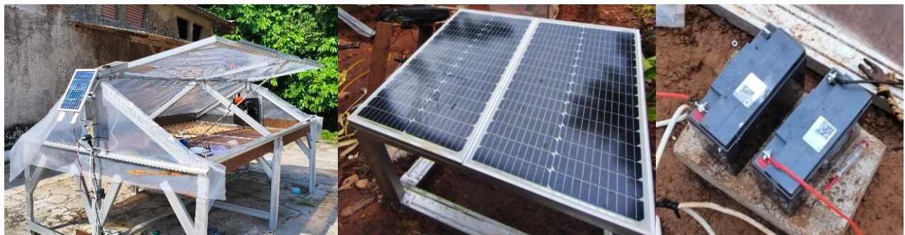
Figure 4. Solar dome dryer, solar PV, and battery
