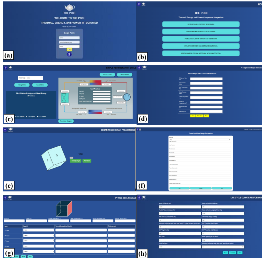
Figure 6. THE POCI Page Preview: (a) Login Page, (b) Main Menu, (c) Performance Analysis Result of Refrigeration System, (d) Parameter Input Form of Module 1, (e) Navigation Page for Cooling Load Calculation, (f) Parameter Input Form of Module 2, (g) Parameter Input of LCCP Module
