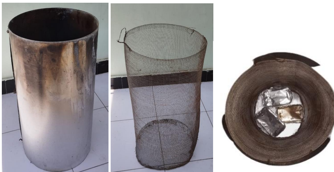
Figure 1. Torrefaction reactor (left), iron basket (middle), and reactor loaded with packed kesambi wastes
