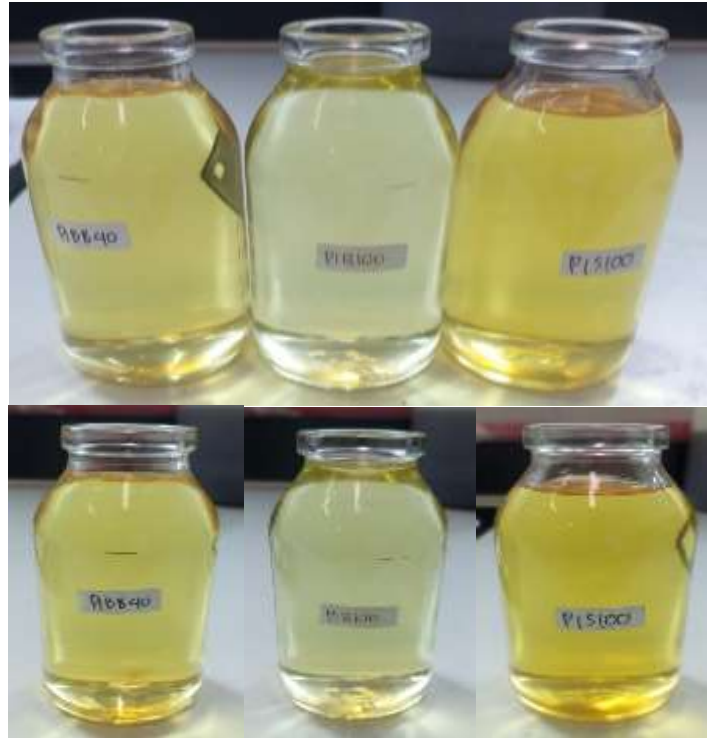
Figure 4. The visual color of fuels, before (top) and after (bottom) storage. (From left: biodiesel mixture B40, neat biodiesel B100, petroleum diesel B0).
