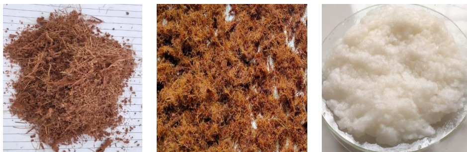
Figure 1. Visual appearance of material: (a) coconut coir, (b) delignified coconut coir, and (c) coconut coir cellulose
