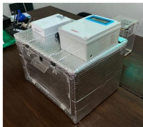
Figure 3. Brown rice germinator: (a) Design, (b) Real germinator. [(1) Box Germinator; 2) Shelves; 3) Mist maker; 4) Water tank; 5) Fan 8 cm x 8 cm; 6) Pipes; 7) Control Box dan LCD Display; 8) Fan 6 cm x 6 cm dan PTC Air Heater; 9) Power Supply]
