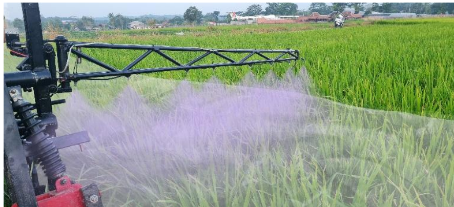
Figure 10. Liquid distribution pattern synchronized with forward speed
