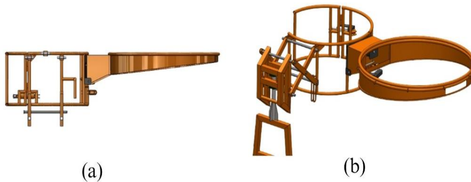
Figure 3. E-Bhar machine FFB catcher components: side view (a), Isometric view (b)
